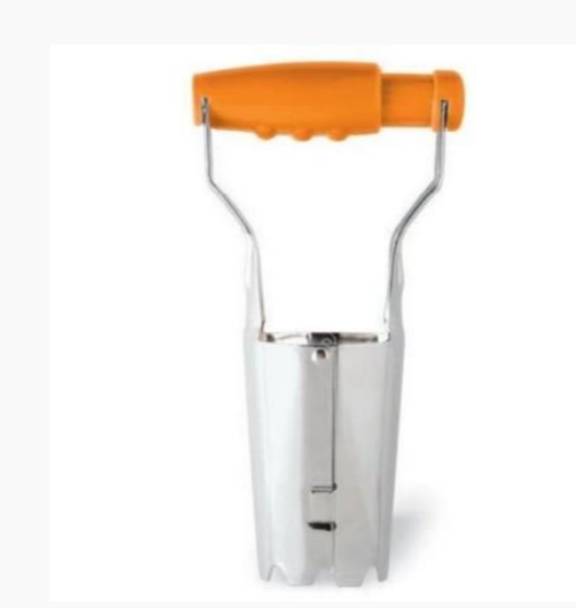
Fig 1: Bulb planter used for undisturbed soil sampling.
