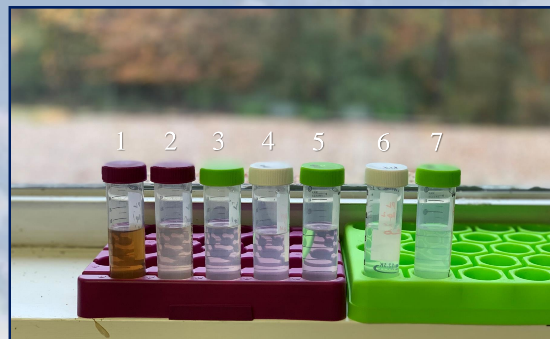
Figure 1: Color variations of the filtrates from the 7-step sequential extraction of poultry litter with de-ionized water.
